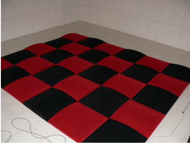
Picture 4: test samples in the reverberation room.
