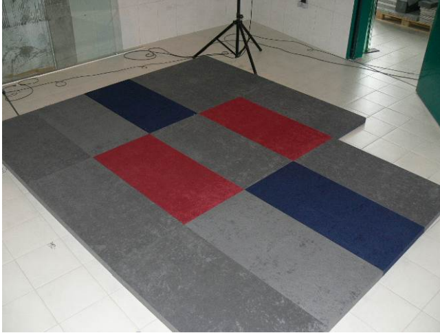
Picture 5: test samples in the reverberation room.
