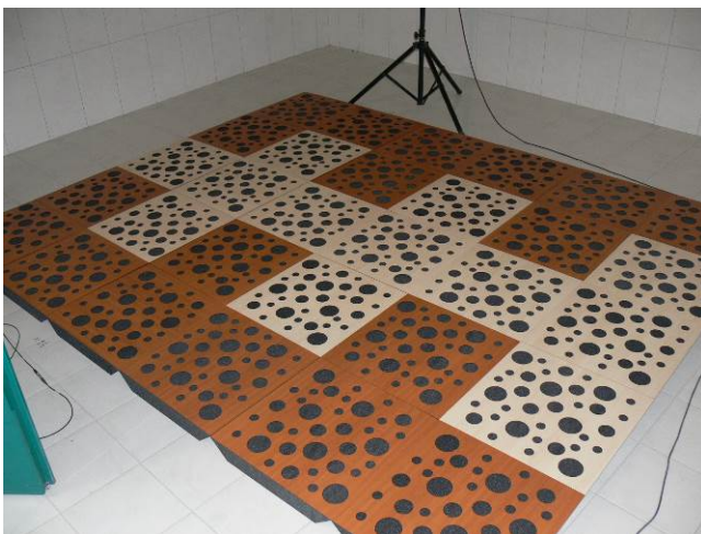
Picture 5: test samples in the reverberation room.
